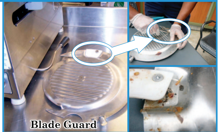
Figure 2. Food soil accumulation on the inside of the blade guard at the white plastic piece.
